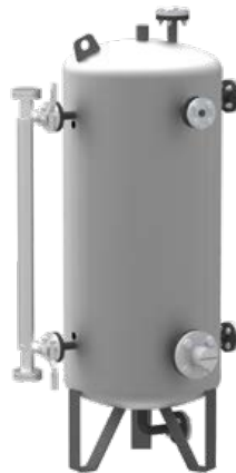
■ Combustion air preheater with smooth pipes, designed to increase the heater efficiency by 4/5%
